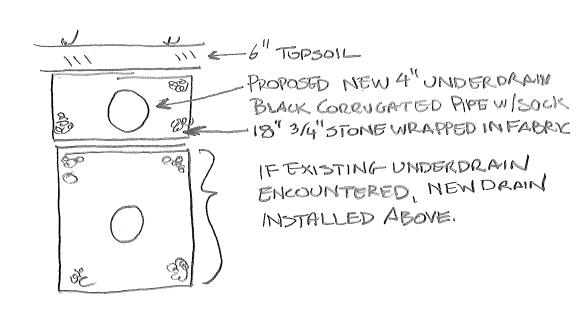
\* NEW 4"UNDERDRAIN PIPE WILL BE TIED INTO ENSTING UNDERDRAIN AT A LOW POINT
